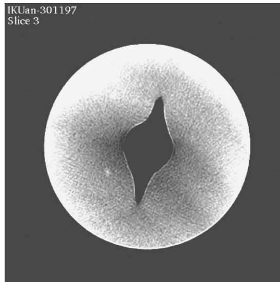
Fig. 19. Borehole breakout configuration in rock (with the courtesy of Papamichos (2002)).
